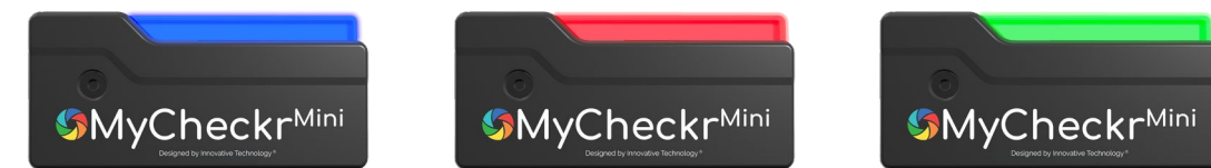
Figure 3: The MyCheckr Mini device illustrating IDLE (Blue), FAIL (Red) and PASS (Green)
