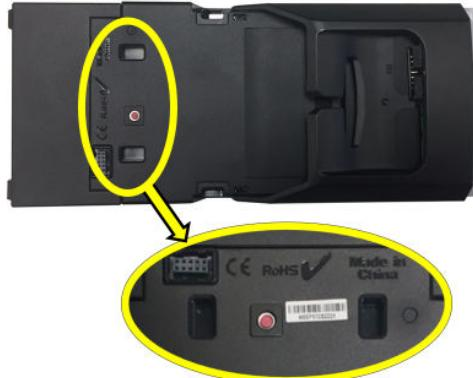
When the internal led starts blinking release the button. The unit will be temporarily in trusted mode when the unit is in ccTalk protocol.
