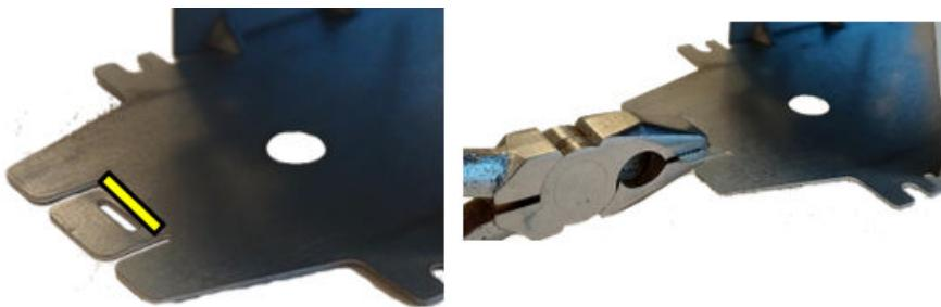
The tab can be fold by hand but if required it can be started with pilers.
