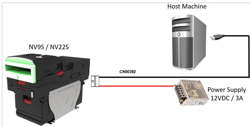
It is not recommended to use IF17 or DA2 (obsolete) to reprogram the device due to the slowness of the data bus which can take up to 20 minutes to update.
