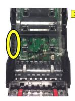
Once the upper housing assembly is lifted, the 16-pin connector socket can be seen on the left-hand side.
