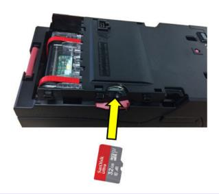
The internal bezel, or rainbow bezel if fitted will flash once when the SD card has been detected.
